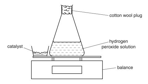
The manganese(IV) oxide is added to the hydrogen peroxide solution and the mass of the flask and contents recorded every 30 seconds. This is **experiment 1**.
